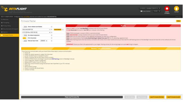
After flashing Bluejay firmware, bidirectional DSHOT can be enabled, and then RPM filtering can be enabled
